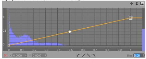
A linear mapping, as shown in the image above, makes color and opacity scale proportional to the input values. In many cases we want to cut off some parts or amplify others, though.
