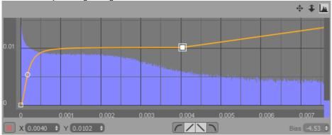
For fire shading, we usually want only a narrow band around the surface of the flame to be visible and luminous. We can do this by defining a small peak in the fire shader's opacity mapping as shown in the image below.
