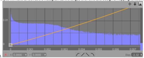
Often it is necessary to create very subtle changes to the mapping function to obtain a certain look. Note the value ranges on the X and Y axes in the image above. The editor has been zoomed in to show the fine details at the low end of the input value range. The histogram shows us that there are still significant changes at this scale and by increasing the intensity for this range (about 0.001 to 0.004) we will get a big visual difference.
